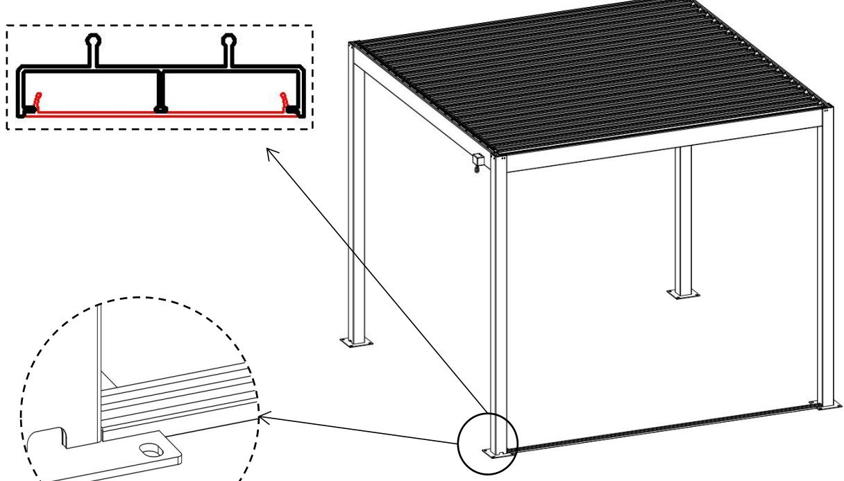
Note: The outside side of B is flush with the outside side of the perloga column
