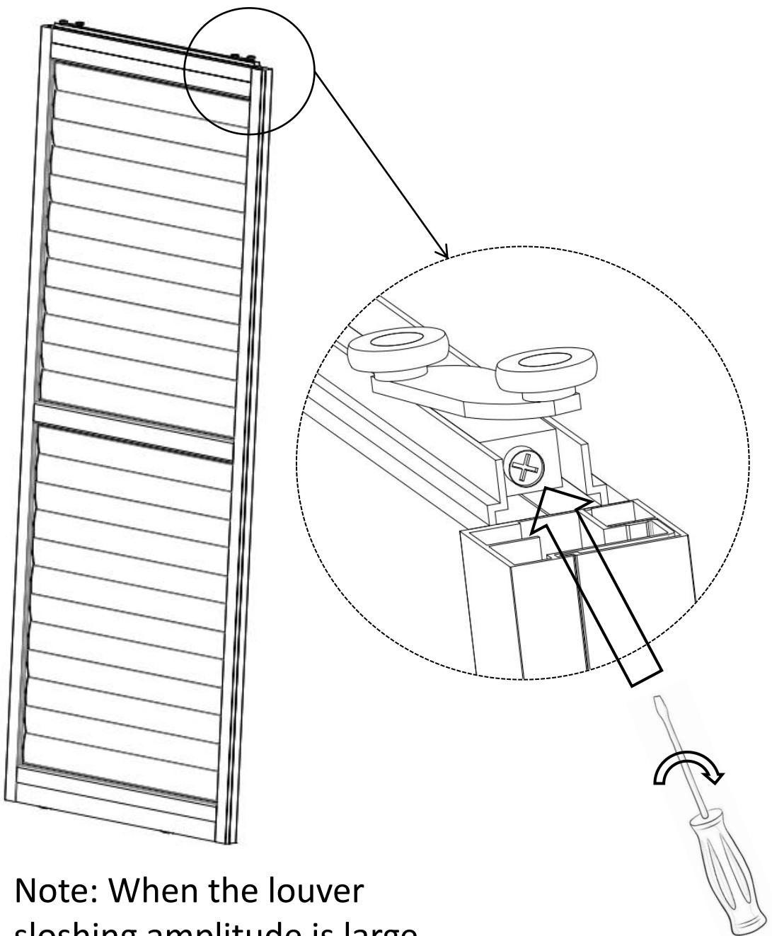
Note: When the louver sloshing amplitude is large after integral installation, the screw of the upper pulley above can be screwed by a Phillips screwdriver to make it more close to the track.
