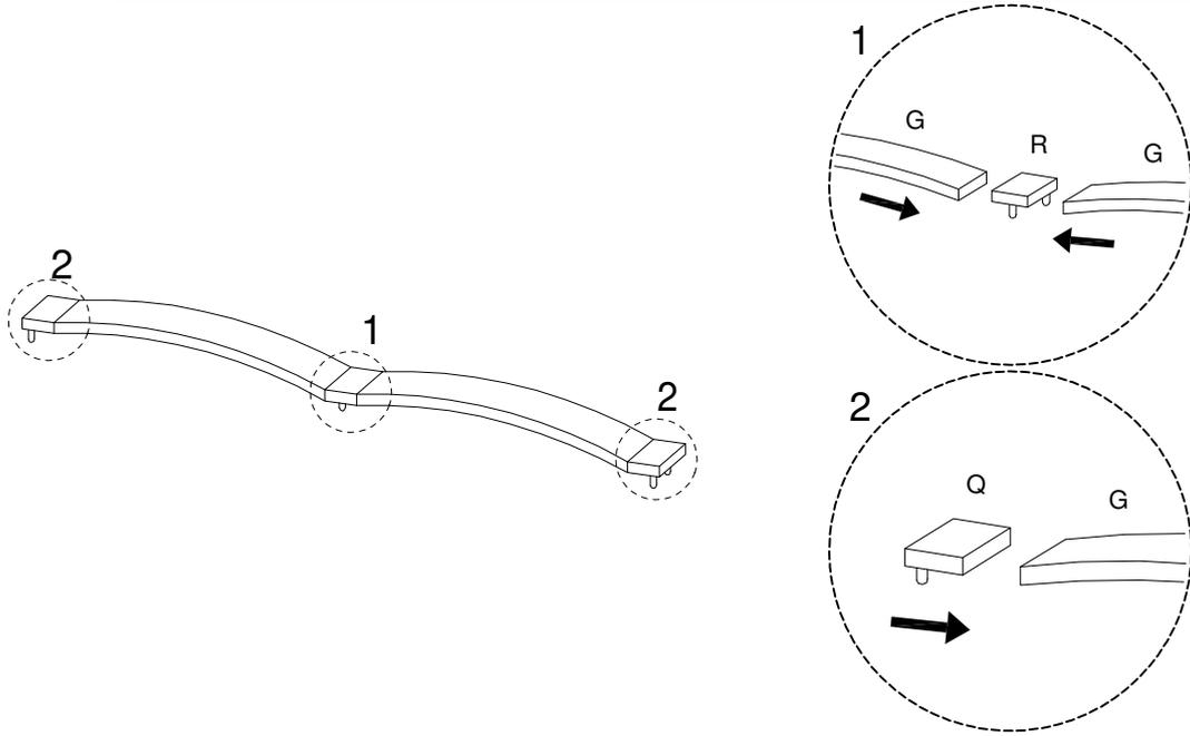
Once the center support feet have been assembled they should be adjusted to ensure they do not touch the floor, 5mm above the floor. When your bed is in place with mattress on top, please adjust the feet so they are in contact with the floor, this will stop any movement.
