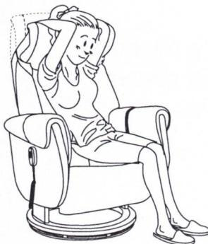
To adjust the headrest, grip the backside of the headrest and pull forward from both sides as shown
