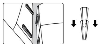
Ensure the two connections on each armrest are all inserted onto the seat tightly.
