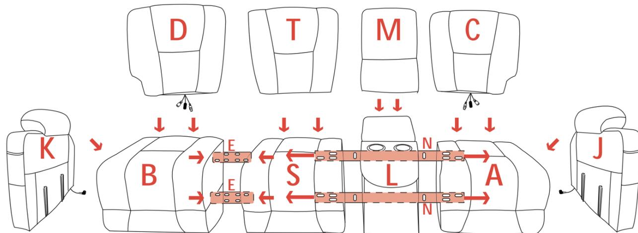
**1.1 Connect part #N to the bases (parts #A, #S) first.**
