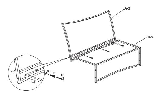
Step 2: Attach the two side panels C&D adjacent to the seat&back panel using bolts F and washer G.
