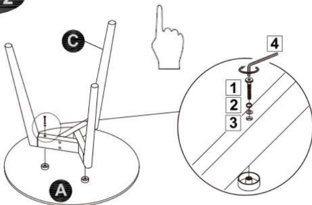
Do not tighten any screw completely until all the screws have been connected.
