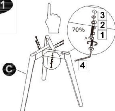
Do not tighten any screw completely until all the screws have been connected.
