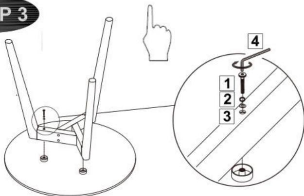
Do not tighten any screw completely until all the screws have been connected.
