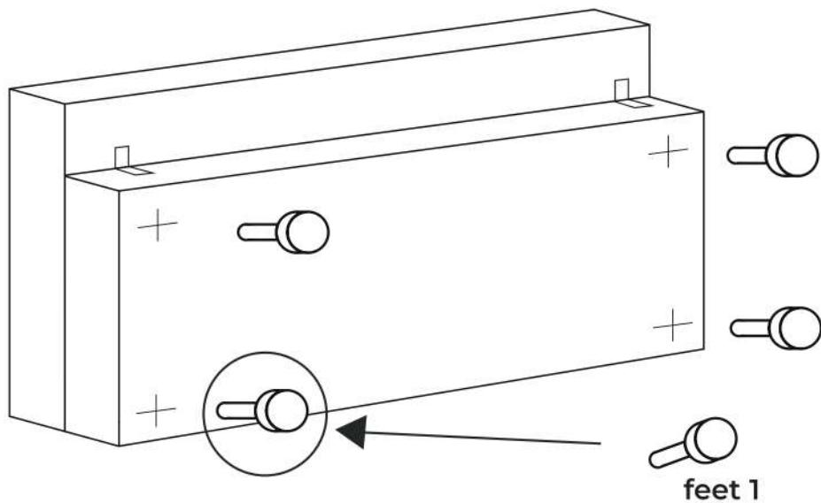
**EN:** And with the screwdriver install the four feets on the marked spots.
