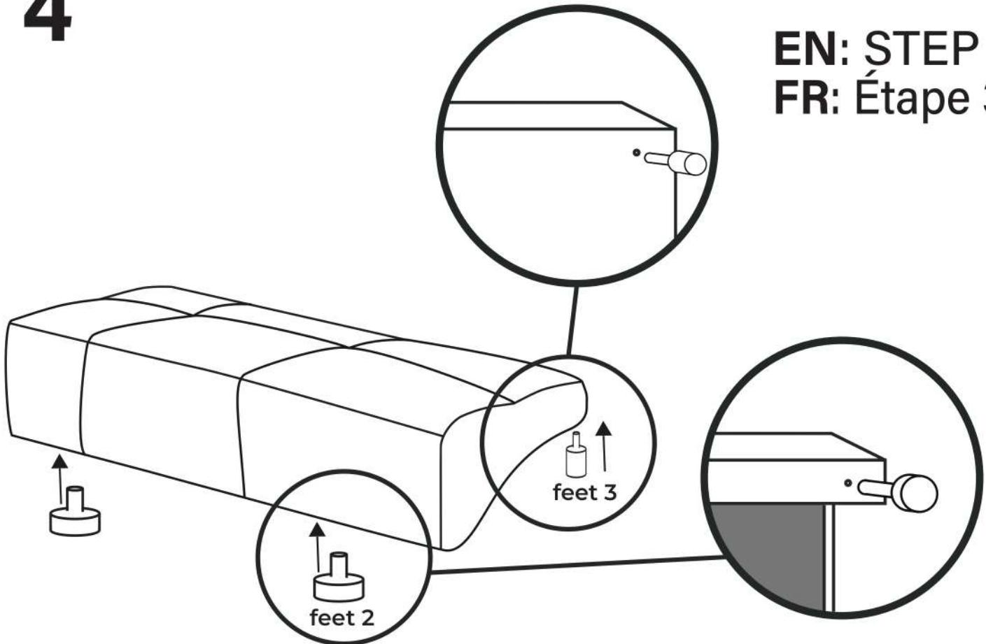
**EN:** Take the sitting part , flip it and install the feets on the marked spots with the screwdriver.
