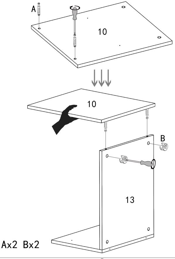
When installing accessories A and B, please refer to the installation method of the same accessories in step 2
